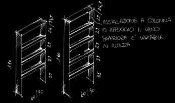
The MODULAR open pantries are a line of accessories designed to increase the functionality of the kitchen work area, through elements in co-extruded aluminium with a burnished finish. Composed of thin sides only 6 mm thick, they are equipped with easily removable and repositionable accessories and are to all intents and purposes a functional alternative to normal shelves, allowing you to have everything in order and close at hand.
